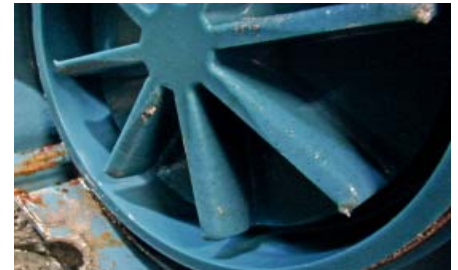
CPRF impeller made of PE 1000R after 7 months
