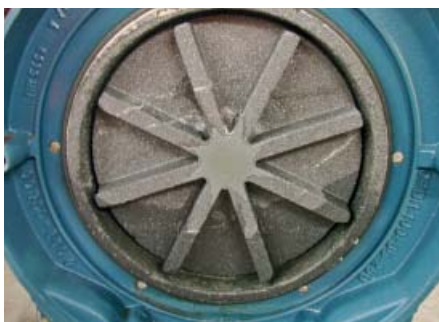
CPRF Impeller made of Polymercarbide after 4 months
