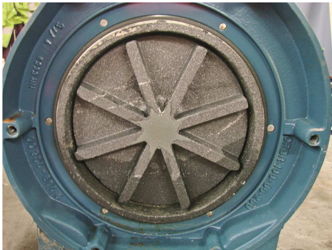
CPRF Impeller made of Polymercarbid after 4 months
