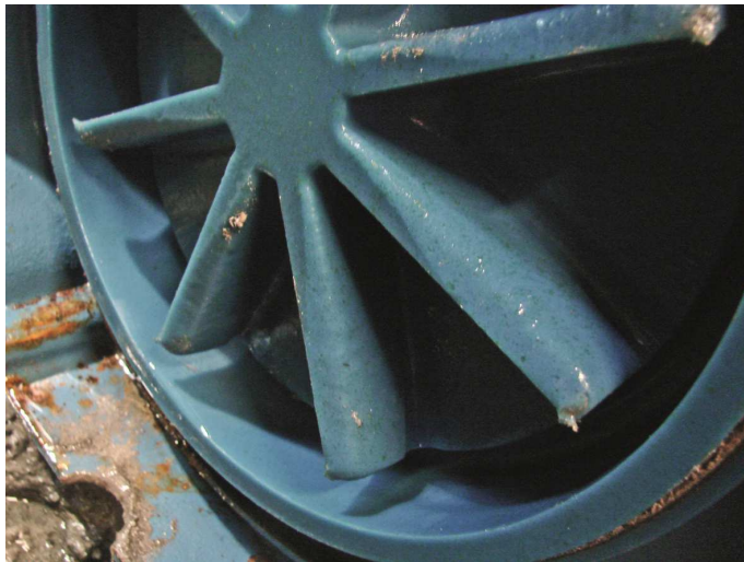
CPRF Impeller made of PE1000R after 7 months
